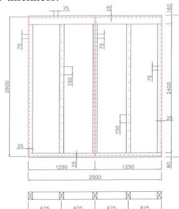
Figure 1: Specimen B12-12 variation drawing
