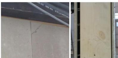
Figure 3: Typical damage and failure mechanism of the panel; cracks of the CPBs (left) and withdrawal of the staples (right)
