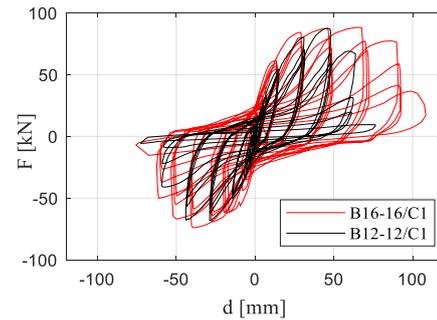
Figure 5: Lateral force-displacement hysteresis curves for panels B12-12 and B16-16 obtained in cyclic tests
