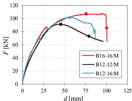
Figure 4: Lateral force-displacement curves for the three types of panels obtained in monotonic tests
